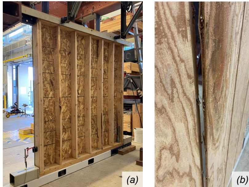
Fig. 7. (a) test wall with OSB sheathing (b) Post-test T1-11 seam with single row of nails.
