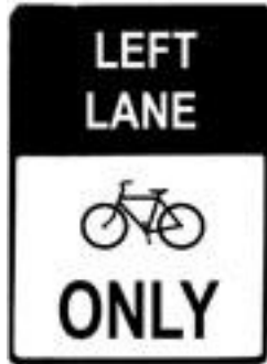
Figure 2: Placed along bike lane (MUTCD R3)
