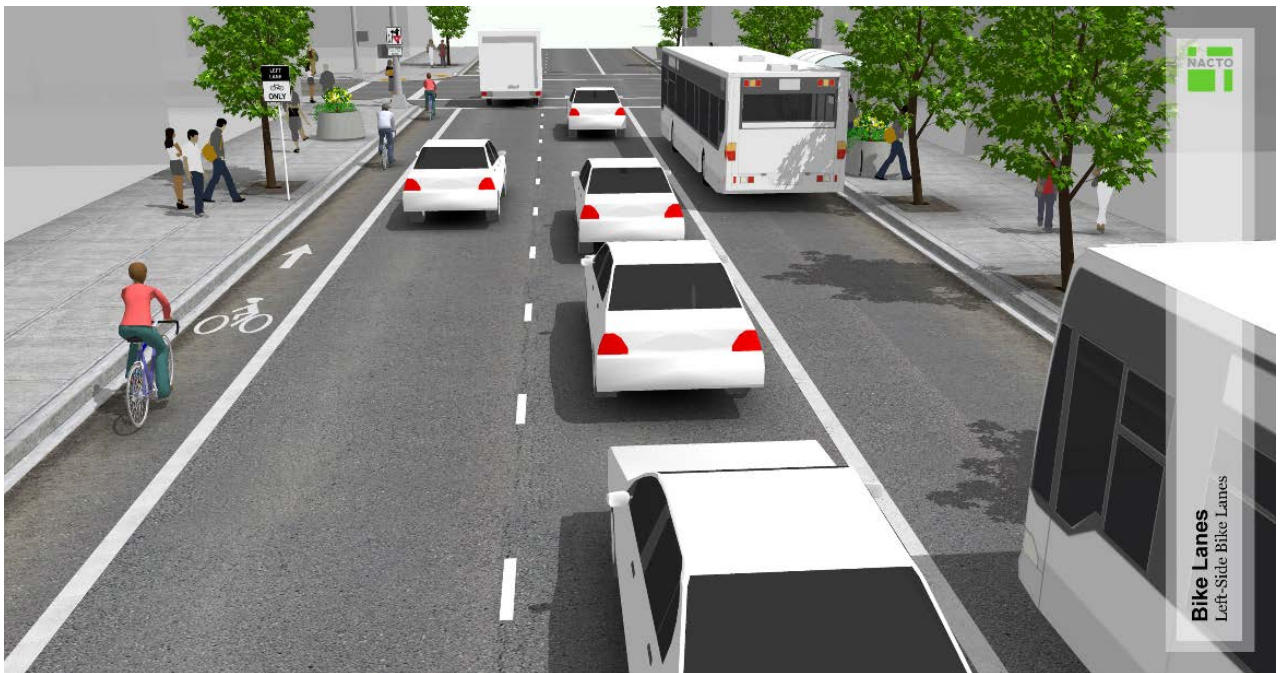
Figure 1: Left Lane bicycle facility courtesy of NACTO
