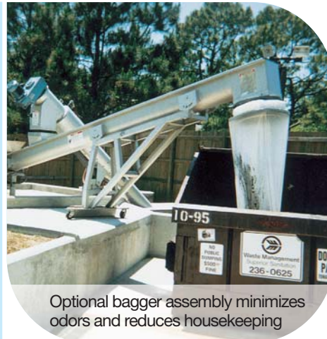
Shaftless conveying spiral provides clear, unrestricted throughput
