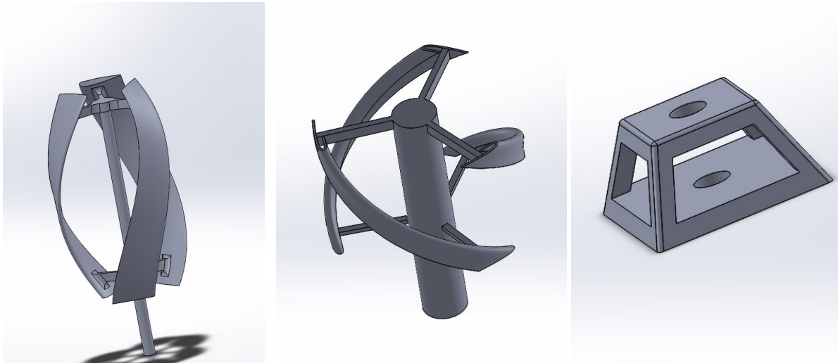
Figure 7. Solid airfoil design (left), Airfoil sheet design (middle), Base (right)
