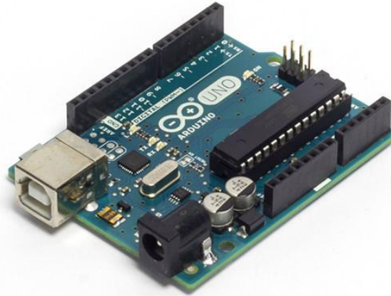
Fig 2.2: The Arduino Uno's small size is a great asset as it allows the control module to be small and unobtrusive.
