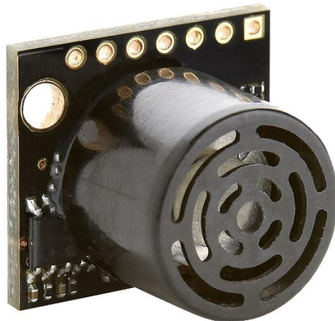
Fig 2.1: A Maxbotix ultrasonic sensor. Depicted is the LV-MaxSonar®-EZ0™ which will be used for the hip component of the system.
