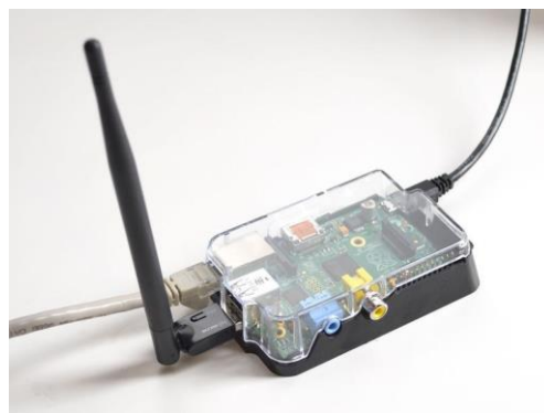
Figure 1.4: Secured Debian Wireless router
