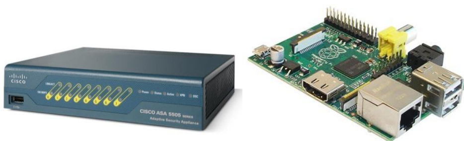
Figure 1.5: Back End components, Gateway firewall and LAMP server
