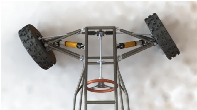
Figure 2. Front suspension and steering.
